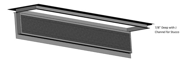
\*Vent shown in open position, Close vent with appropriate fasteners (min. 3) along the front nail flange
